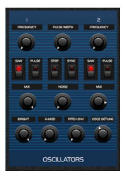
A mixer was introduced to blend the two oscillators and noise source which is much more flexible than the fixed levels of the original design.
