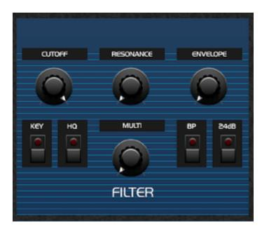
It implements a Multimode 12dB/ octave filter like the Oberheim SEM module. Using the **MULTI** rotary control, you can crossfade between low-pass behavior on the complete left, to either notch (by default) or bandpass (using the BP switch) behavior at 12 o'clock, and high- pass behavior on the far right.
